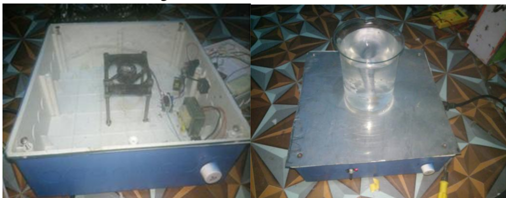
Fig. 13 The Constructed Magnetic Stirrer
