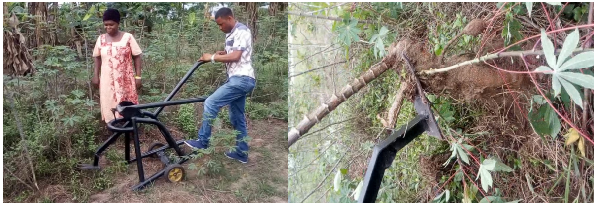
Figure 8: Field trial pictures to showcase the operation of the manual Cassava Harvester.
