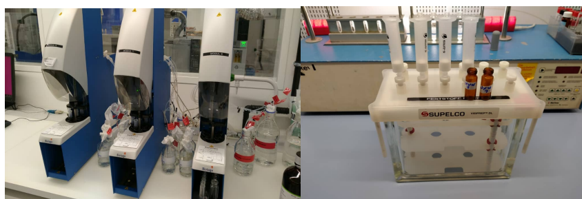
Figure1: An automated SPE Extractor Figure2: A traditional manifold SPE Techniques
