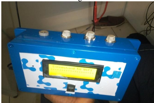
Figure 10: Pictorial view of the developed real-time web-based air quality monitoring system
