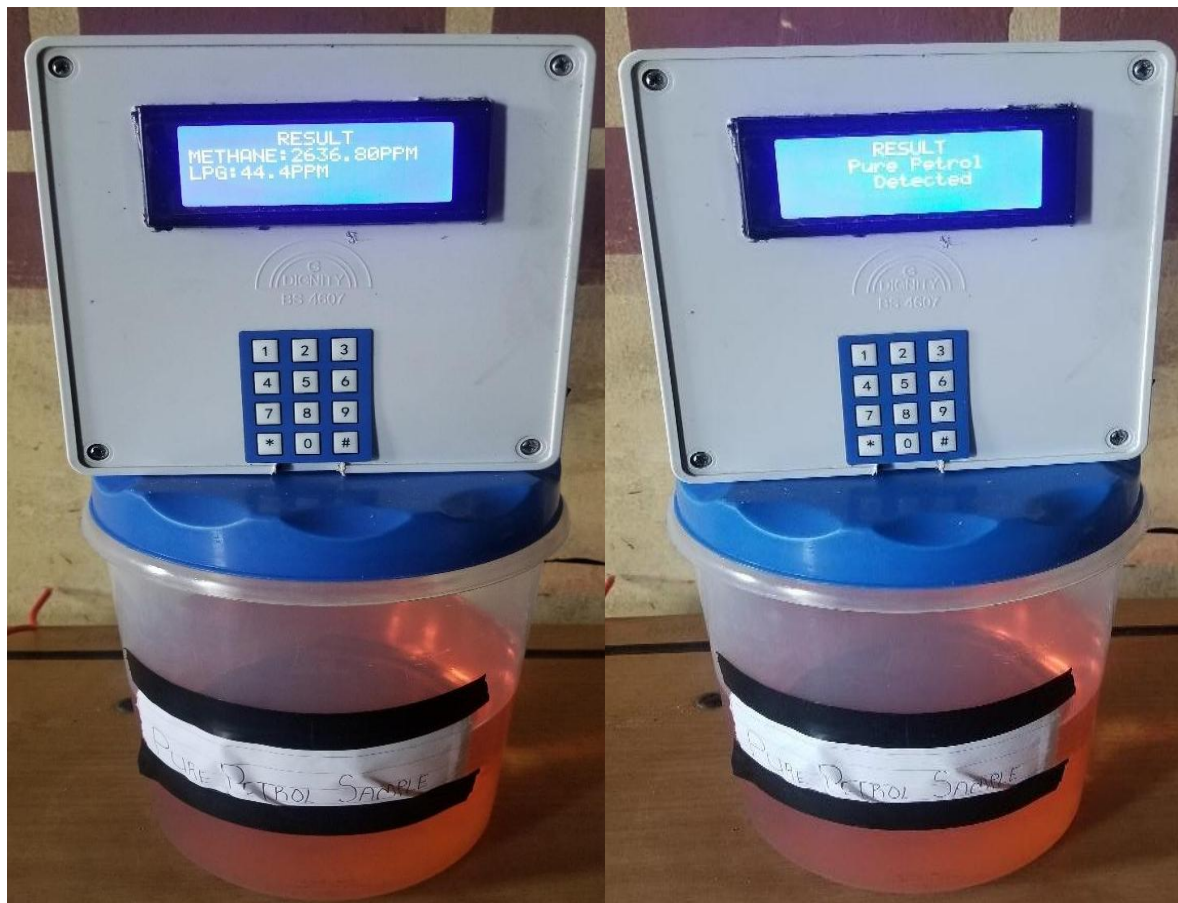
(a) Test result showing concentration of gases of pure petrol sample
