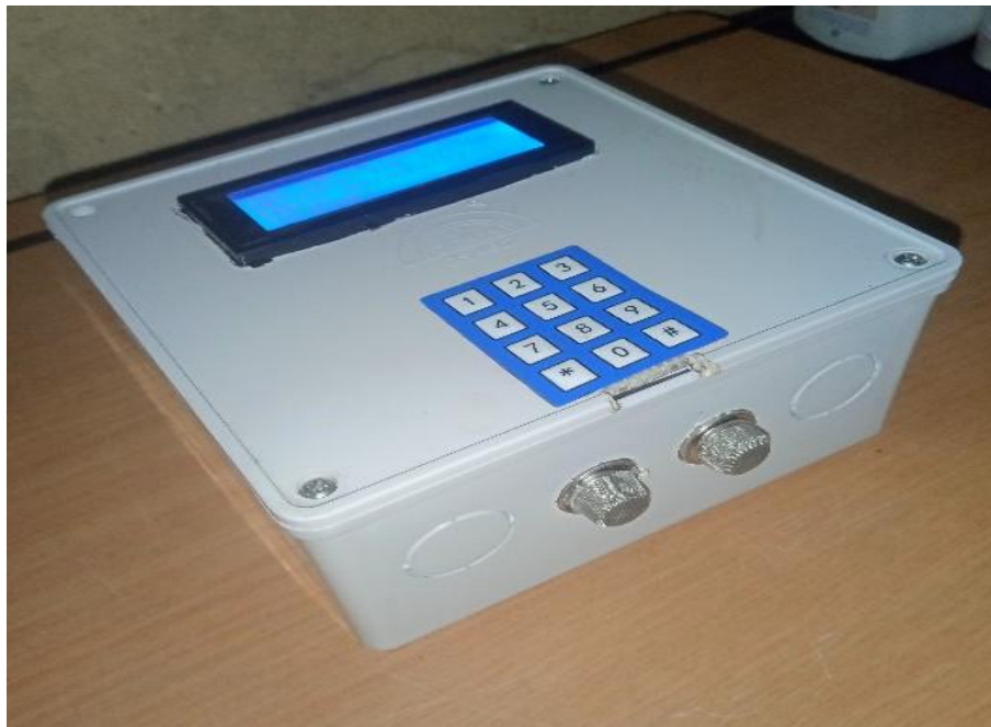
Fig. 7: Constructed electronic device for detecting adulteration of petroleum products
