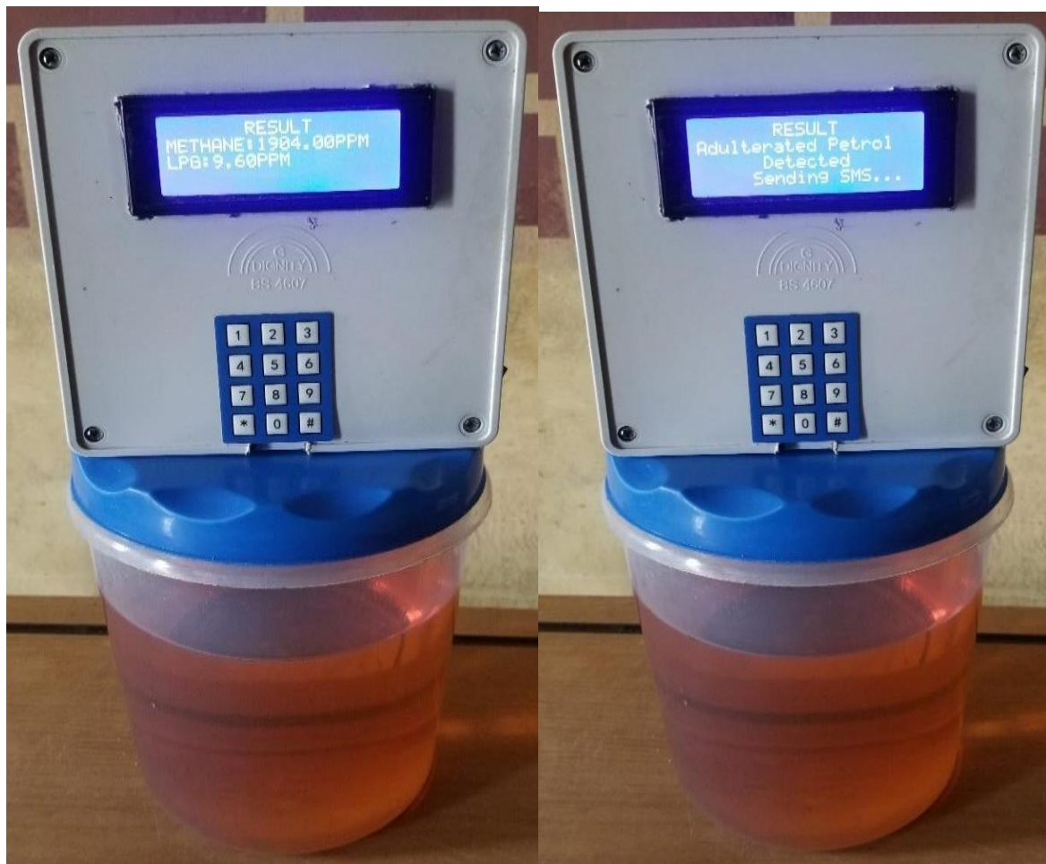
(b) Test result indicating detection of adulterated petrol sample
