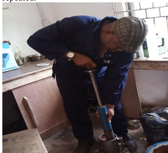
Plate 4: Compaction test on the soil samples
