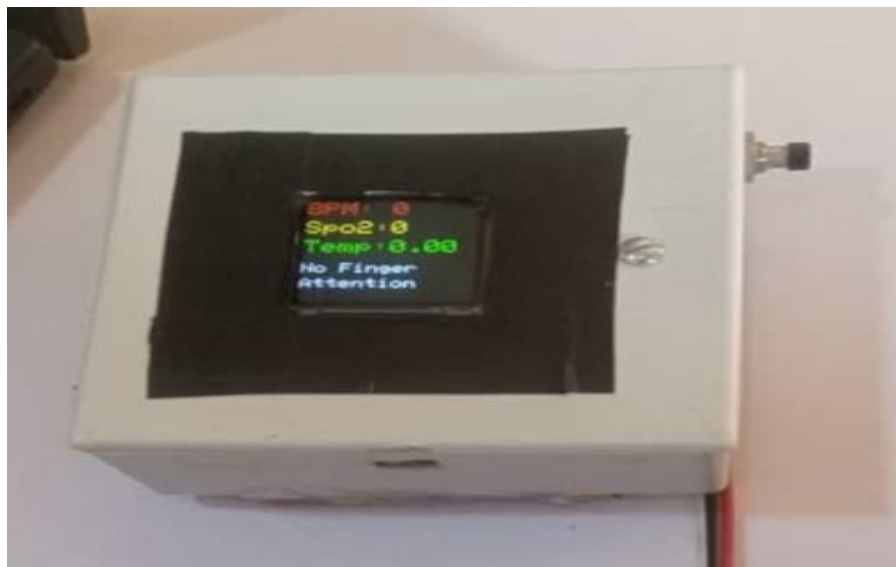
Figure 10: Pictorial view of the IoT-based device connected to the internet with no finger placed on the sensor (Source: Author)
