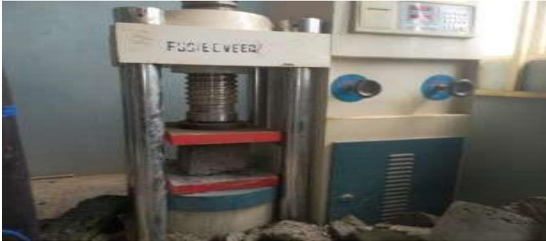
Figure 5: Crushing of concrete cubes.
