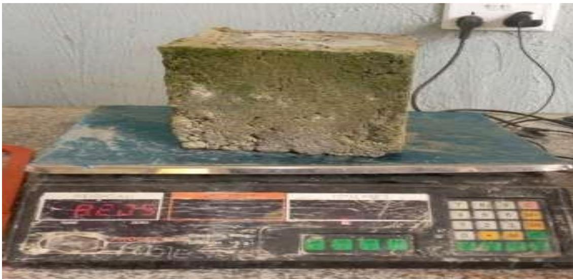
Figure 6: Weighing of concrete cube for density determination.
