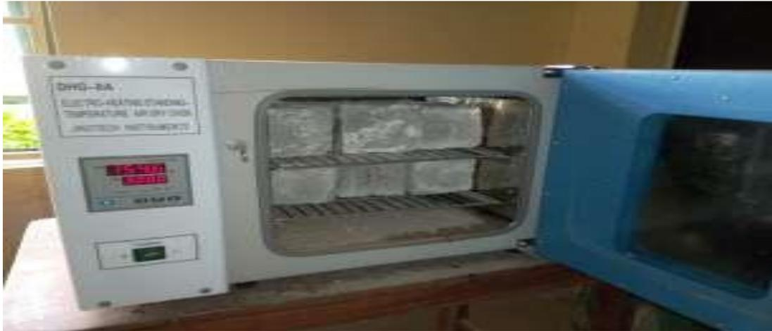
Figure 3: Drying of concrete specimen in an oven.
