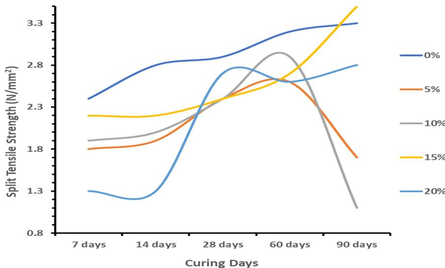
Figure 9: Splitting Tensile strength graph.
