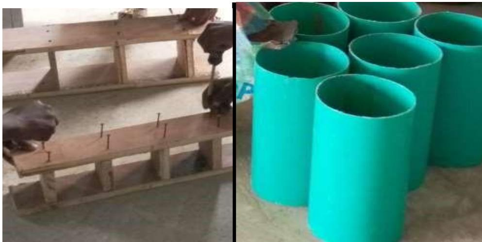
Figure 1: Wooden moulds and P.V.C cylindrical moulds (pipes)
