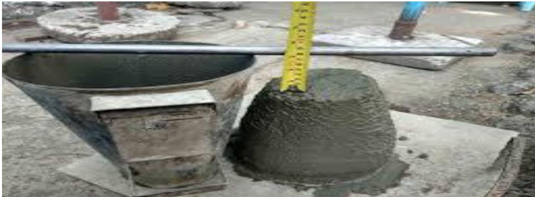
Figure 2: Slump test
