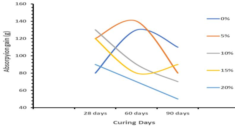
Figure 10: Water absorption graph
