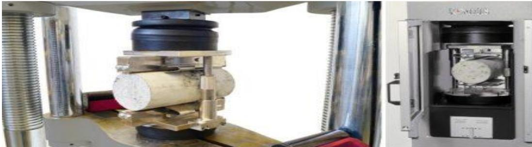
Figure 7: Splitting tensile test of concrete specimen.
