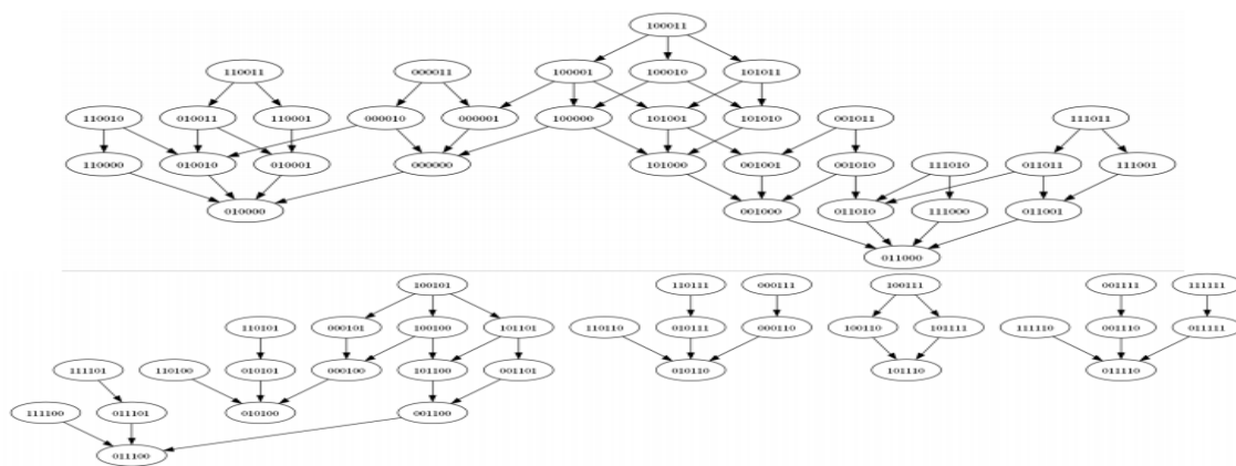
Figure 5: State transition graph of the reduced Life kinetics and Impairment Network (Parameters are encoded in the following order: {mci, meanws, numfir, ttib, waso, wscv})
