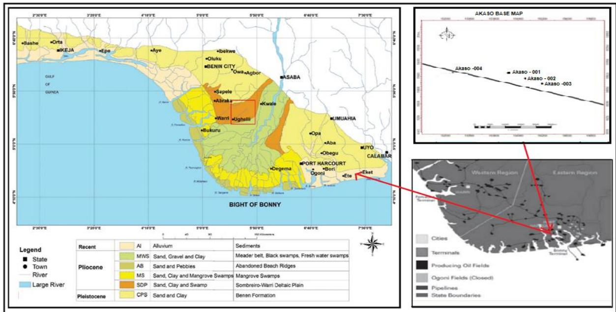
**Figure 1: Basemap of Osaka Field showing the relative position of the wells within the field and their location in the Niger Delta sedimentary basin**
