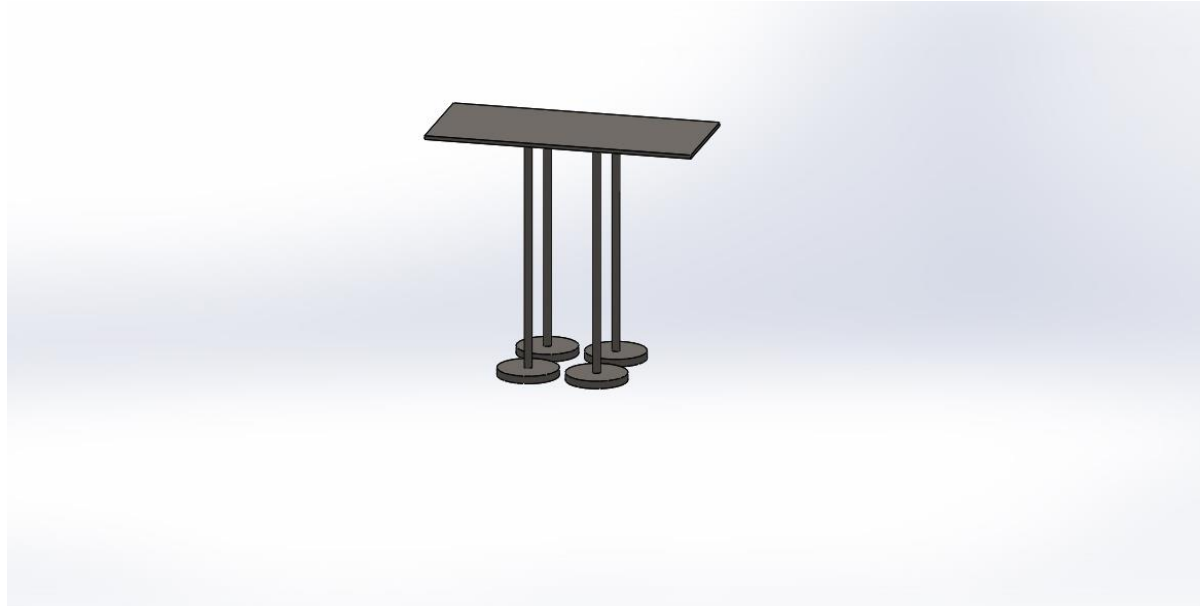
Figure 3. Piston and compression plate of the briquetting machine.
