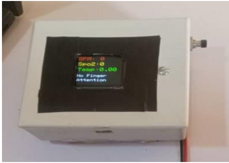
Figure 10: Pictorial view of the IoT-based device connected to the internet with no finger placed on the sensor (Source: Author)
