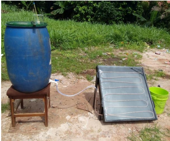
Figure 1: Experimental setup of the flat plate solar collector
