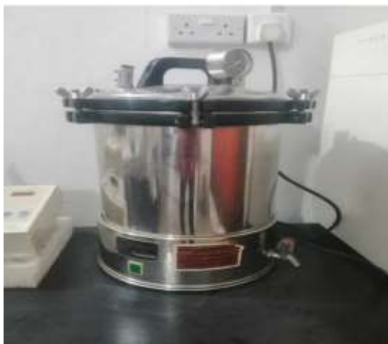
Figure 4. Autoclave: sterilization of agar nutrient to kill microorganisms
