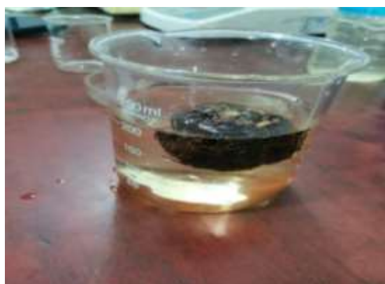
Figure 3: Sample of Cow dung designed to float at specific depth and water density
