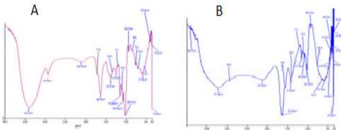
**Figure 1:** FTIR Spectra of (A) ACS and (b) CMS before metal adsorption
