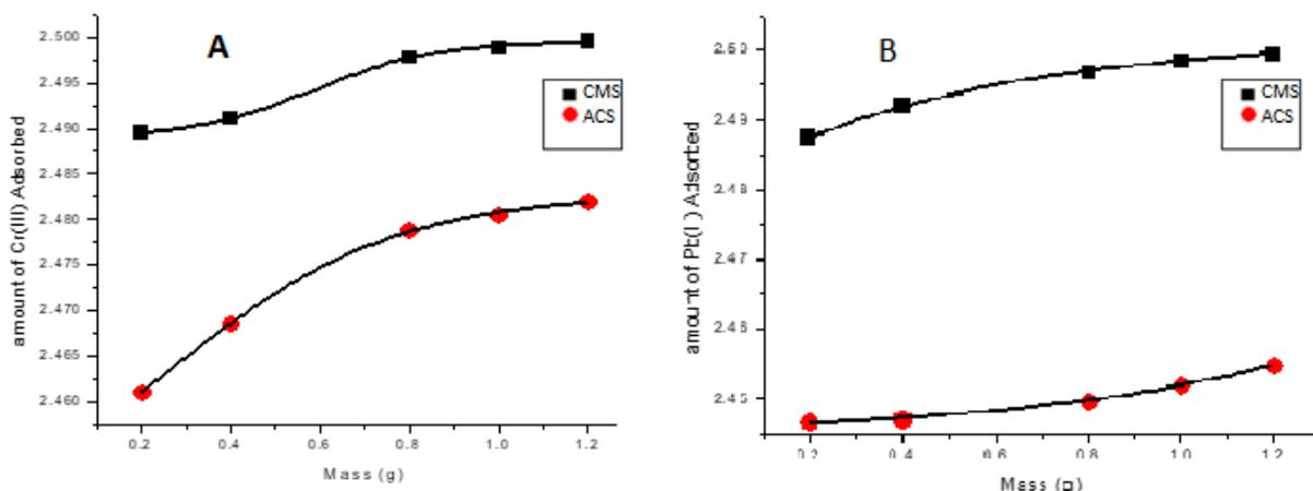
**Figure 5:** Effect of initial adsorbent dosage on adsorption of (A) Cr<sup>3+</sup> and (B) Pb<sup>2+</sup>
