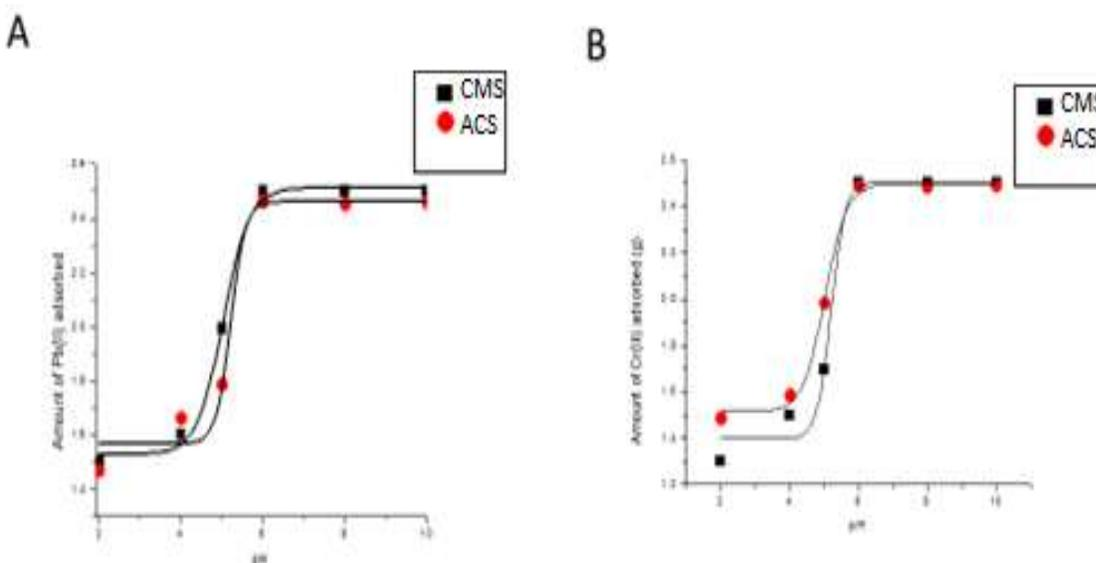
**Figure 3:** Effect of pH on adsorption of (A)  $\text{Cr}^{3+}$  and (B)  $\text{Pb}^{2+}$
