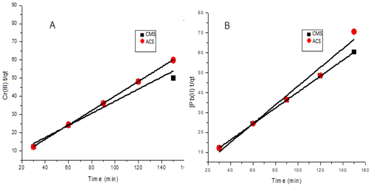
**Figure 10:** Pseudo-second-order plot for the adsorption of (A) Cr<sup>3+</sup> and (B) Pb<sup>2+</sup>
