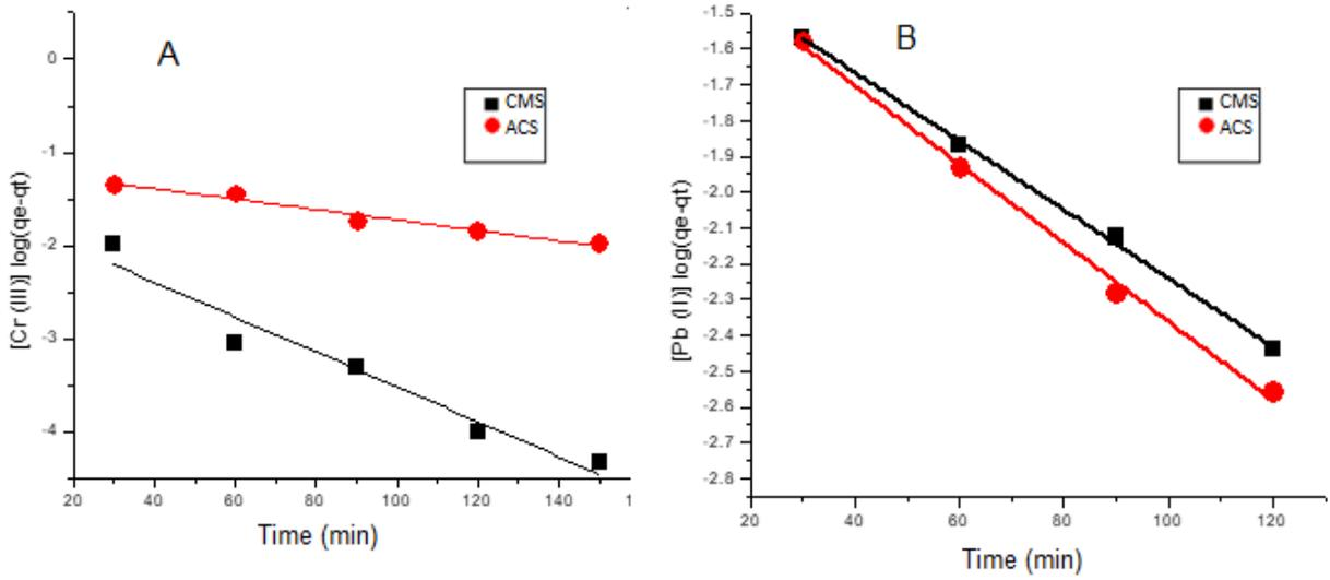
**Figure 9:** Pseudo-first-order plot for the adsorption of (A) Cr<sup>3+</sup> and (B) Pb<sup>2+</sup>
