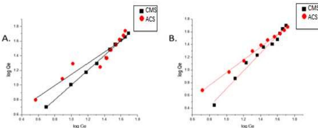
**Figure 8:** Freundlich Isotherm for the adsorption of (A)  $Cr^{3+}$  and (B)  $Pb^{2+}$
