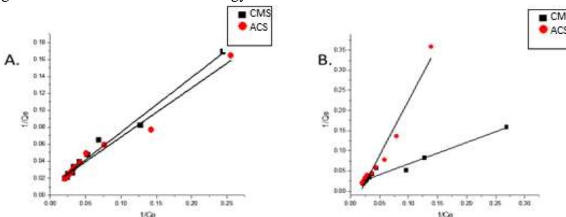
**Figure 7:** Langmuir Isotherm for the adsorption of (A)  $Cr^{3+}$  and (B)  $Pb^{2+}$
