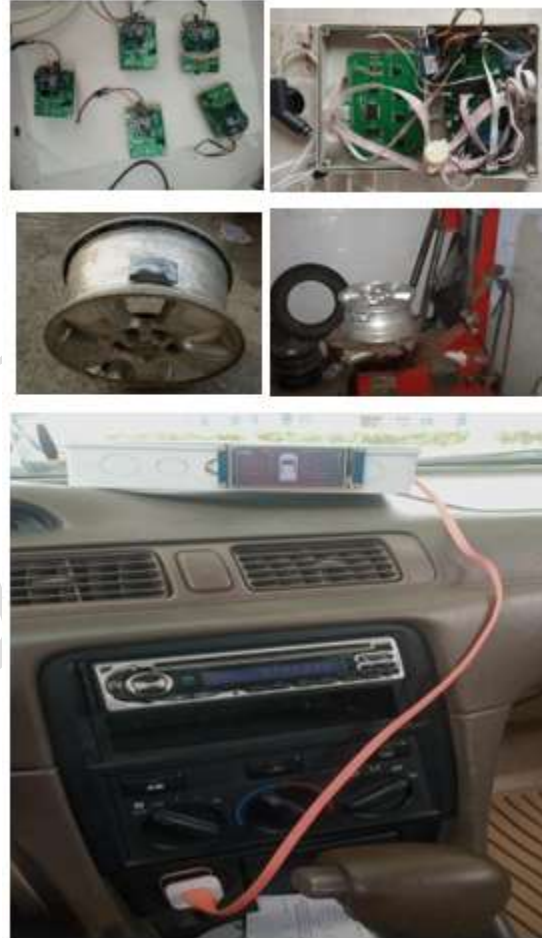
Figure 8: Implementation and installation of the developed TPMS
