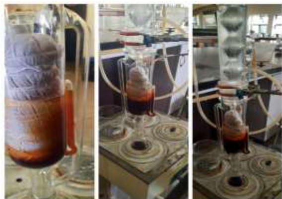
Plate 2.3 (a), (b) and (c): An image of the extraction of the solvent using the Soxhlet extractor
