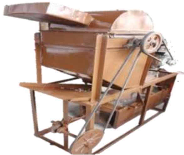
Figure 11: Picture view of the fabricated groundnut shelling machine
