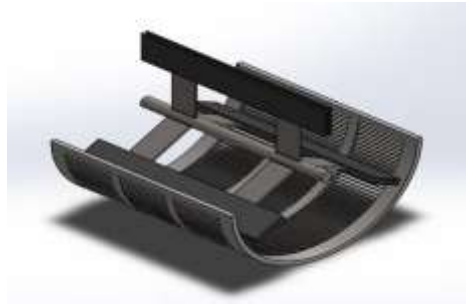
Figure 3: The CAD model of the shelling chamber arrangement
