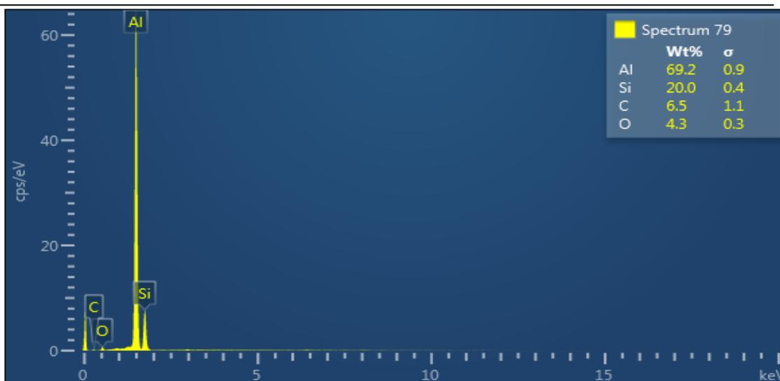
**Figure 7. EDS Spectrum of point 79**
