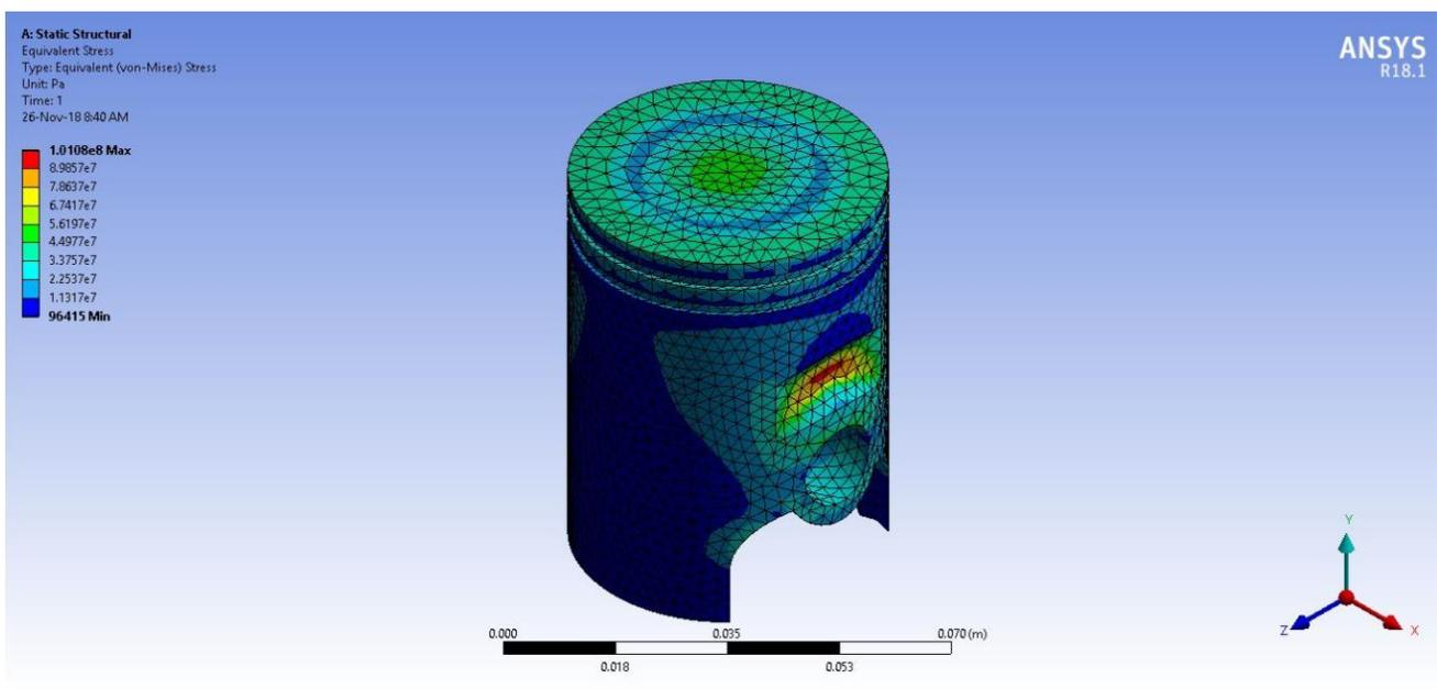
Figure 11. von Mises stress distribution
