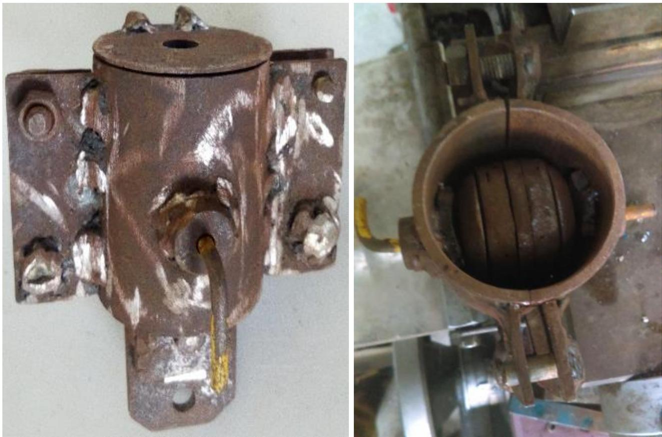
**Figure 2. The permanent mould developed from AISI 1018 steel**
