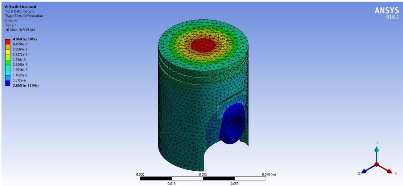
**Figure 12. The total deformation of the piston**
