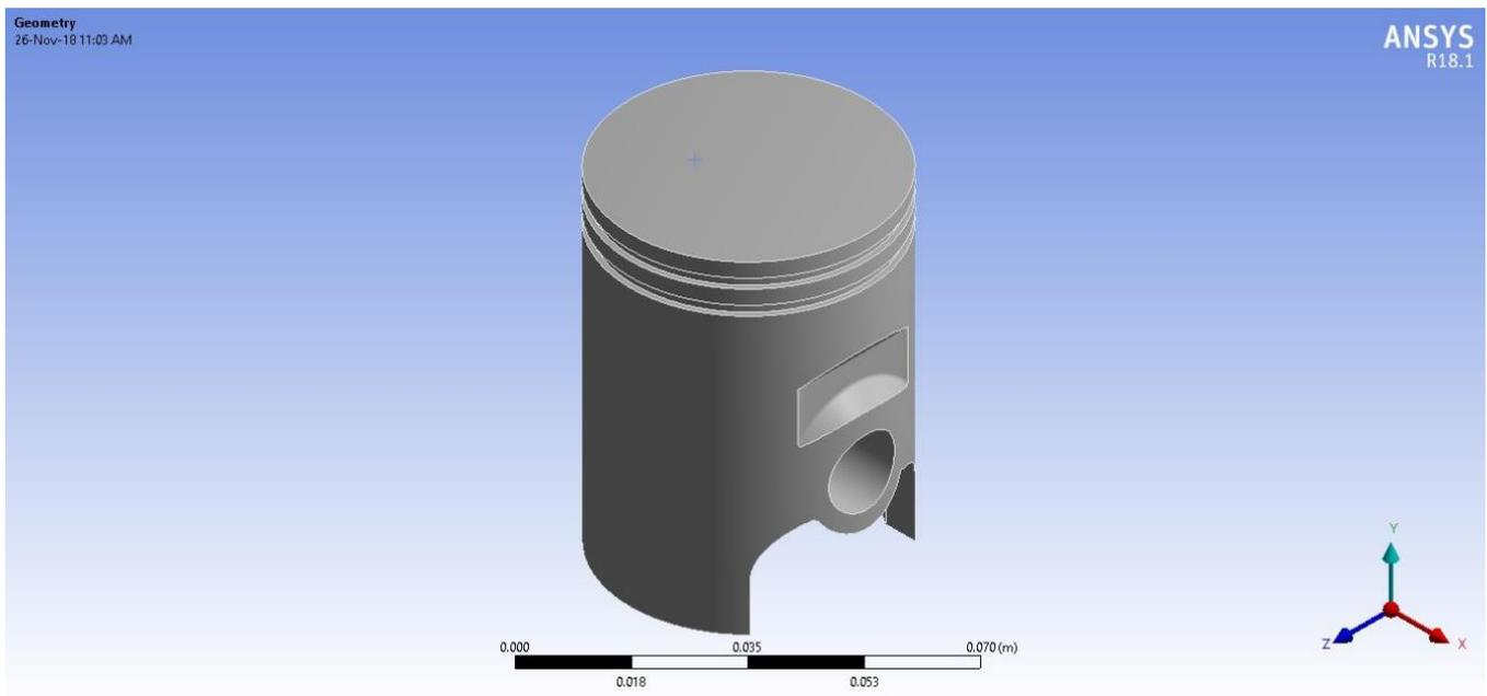
**Figure 4. CAD geometry of the aluminium piston**
