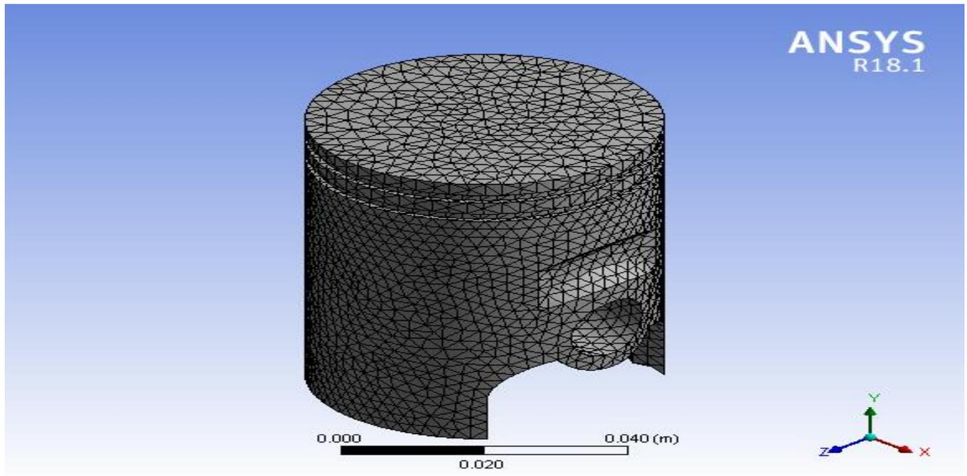
**Figure 5. Discretised aluminium piston with 35573 nodes and 20441 elements**
