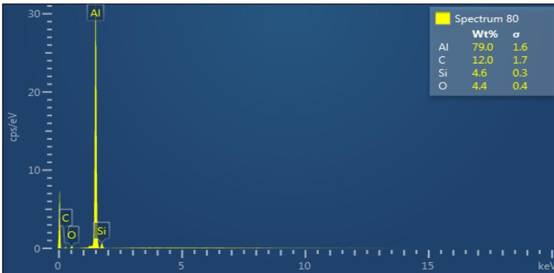
Figure 8. EDS Spectrum of point 80
