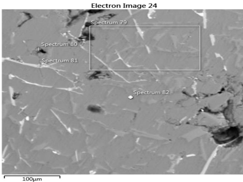
**Figure 6. SEM-EDS micrograph of Aluminum displaying points of interest**
