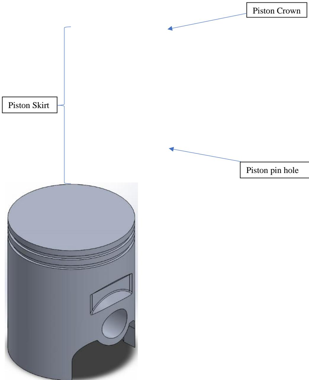
**Figure 1. Parts of a Piston**
