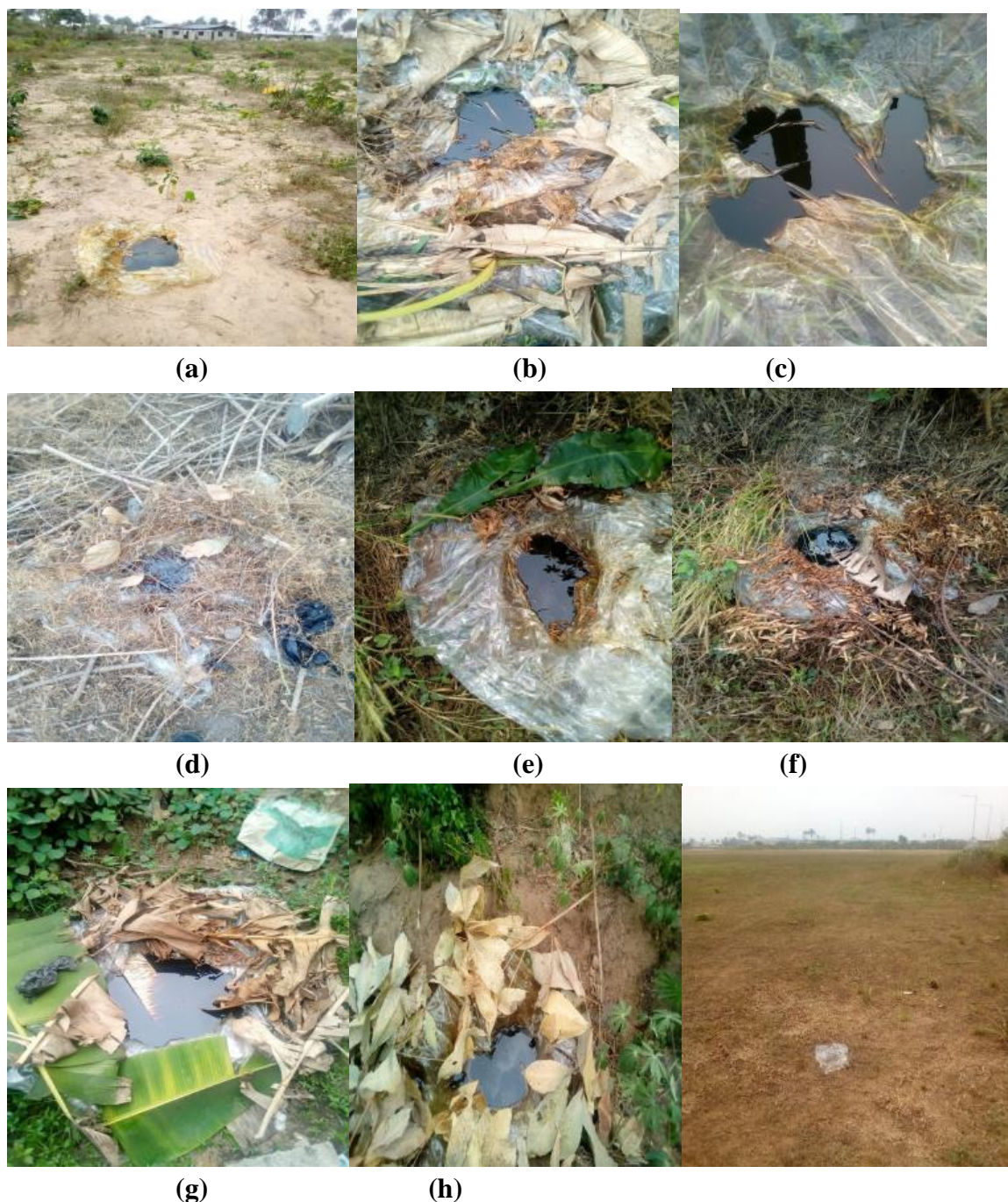
Figure 4: Ground Truth Crude Oil Visible Images from the Crude Oil Spill Imaging Database. (a) Image_0102: Day Image, Volume: 0.5 L, Surface Area: 43 cm x 37 cm (b) Image_0021: Day Image, Volume: 1 L, Surface Area: 40 x 32 cm (c) Image_0012: Day Image, Volume: 1 L, Surface Area: 49 x 48 cm (d) Image_0029: Day Image, Volume: 0.5 L, Surface Area: 22 x 22 cm (e) Image_0088: Day Image, Volume: 1 L, Surface Area: 23 cm x 27 cm (f) Image_0083: Day Image, Volume: 2 L, Surface Area: 31 cm x 38 cm (g) Image_0078: Day Image, Volume: 3 L, Shape: Circular, Diameter: 55 cm (h) Image_0063: Day Image, Volume: 3 L, Surface Area: 49 cm x 35 cm (i) Image_0039: Day Image, Volume: 0.01 L, Surface Area: 6 cm x 6 cm
