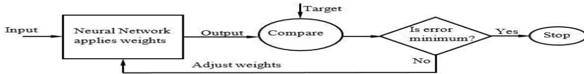
Fig. 2: Flow chart for training the neural network of oil and gas pipeline corrosion rate
