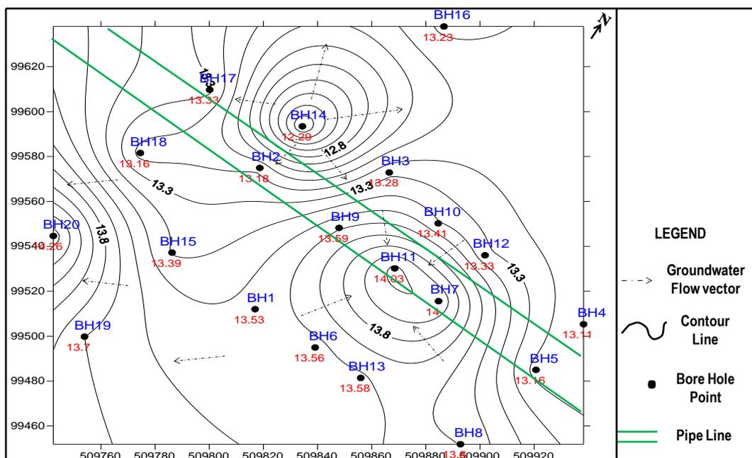
Fig. 6: Top Groundwater level contour map at the site
